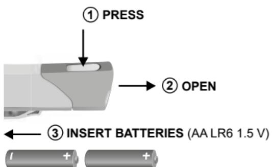
To change the batteries, the battery cap must be removed and refitted after inserting the batteries (see illustration).
